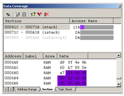
Figure 5.117 Data Coverage window (section name specification)
